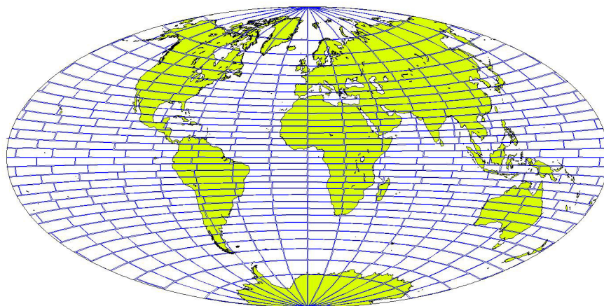
Figure 2.7 2D partitioning, for 512 MPI tasks.
