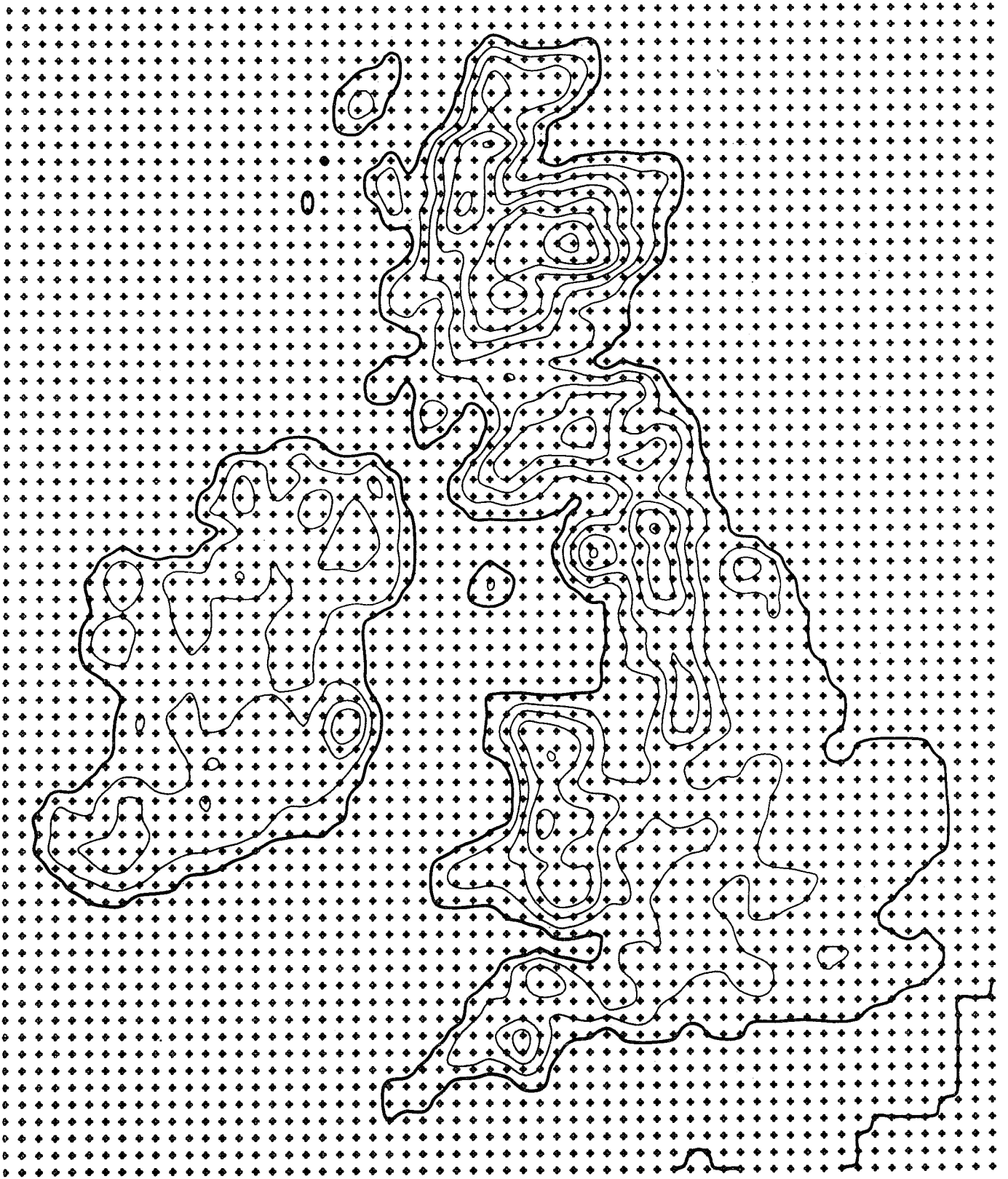
Fig. 1 Domain and orography currently used for mesoscale forecasts. The contour interval is 100 m and the gridlength is 15 km.
