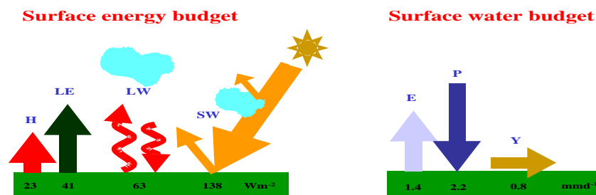
Figure 1. Schematics of surface energy and water fluxes. H , LE , LW and SW stand for surface sensible and latent heat flux, surface longwave and shortwave radiation flux, respectively; E , P , and Y stand for evaporation, precipitation and runoff. Numbers at the bottom represent averaged values over all land points for the ERA15 reanalysis (1979–1993).
