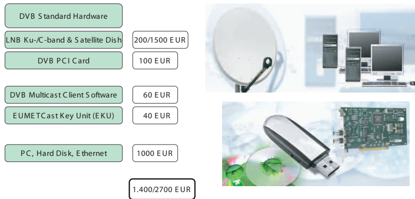
Fig. 4 GEONETCast reception system (variations might be possible depending on GNC operator)
