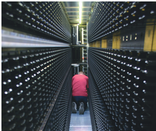
Figure 3 Inside one of the two corridors of an SL8500. Each ATL can house up to 10,000 tape cartridges.
