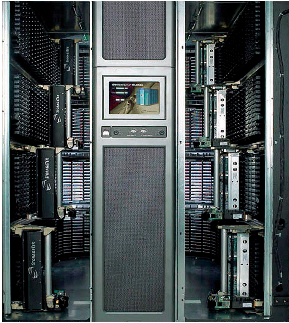
Figure 5 The eight 'handbots', four in each corridor and two on each rail.
