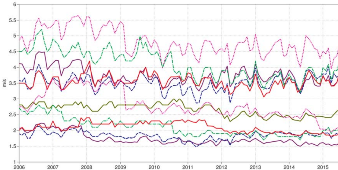
Figure 16: WMO-exchanged scores from global forecast centres. RMS vector wind error over tropics at 250 hPa (top) and 850 hPa (bottom). In each panel the upper curves show the five-day forecast error and the lower curves show the one-day forecast error. Each model is verified against its own analysis.
