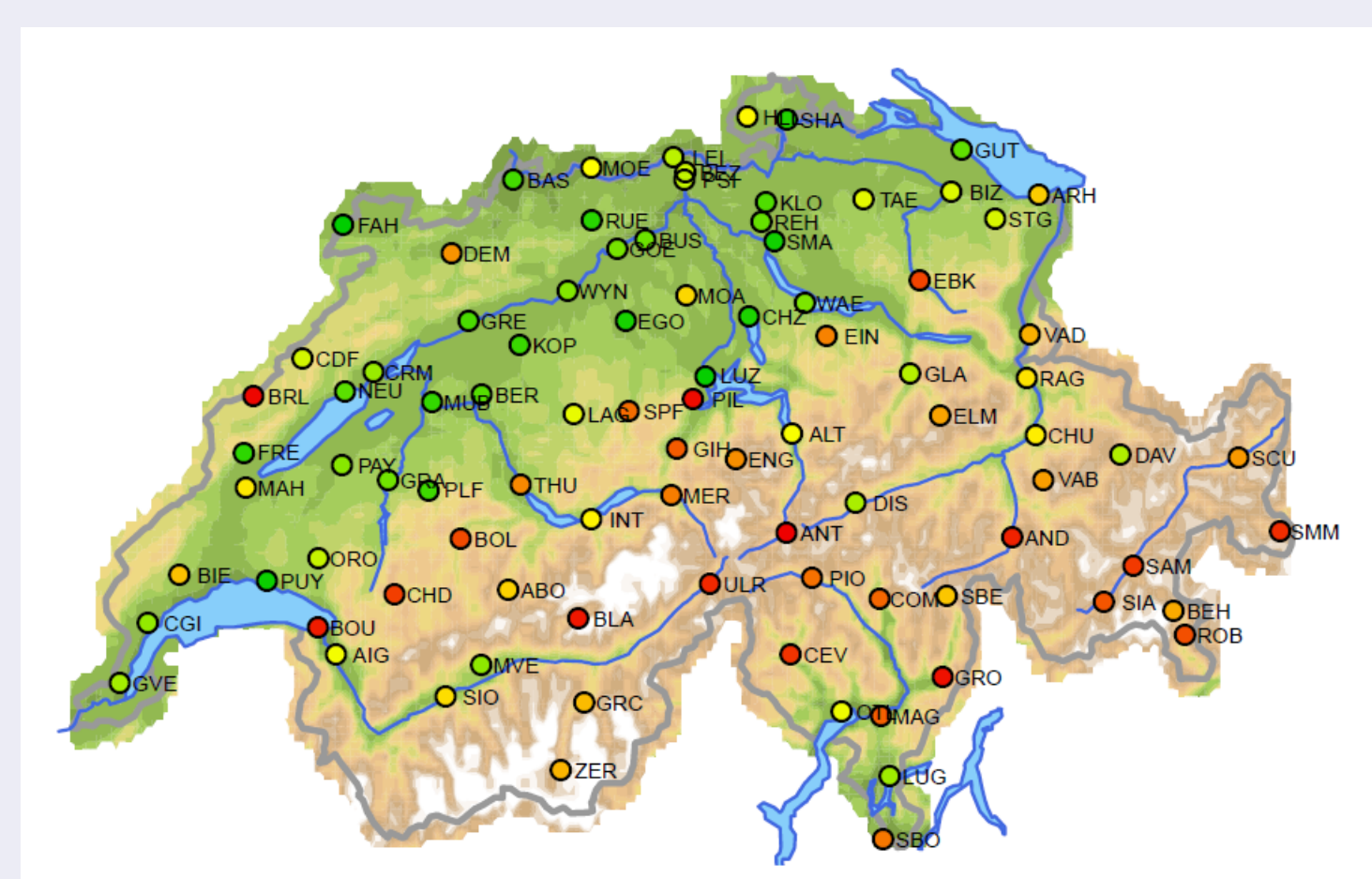
Figure 4: 2m temperature verification for 2015. Stations are ranked according to mean absolute error. Green for top rank, red for low.
