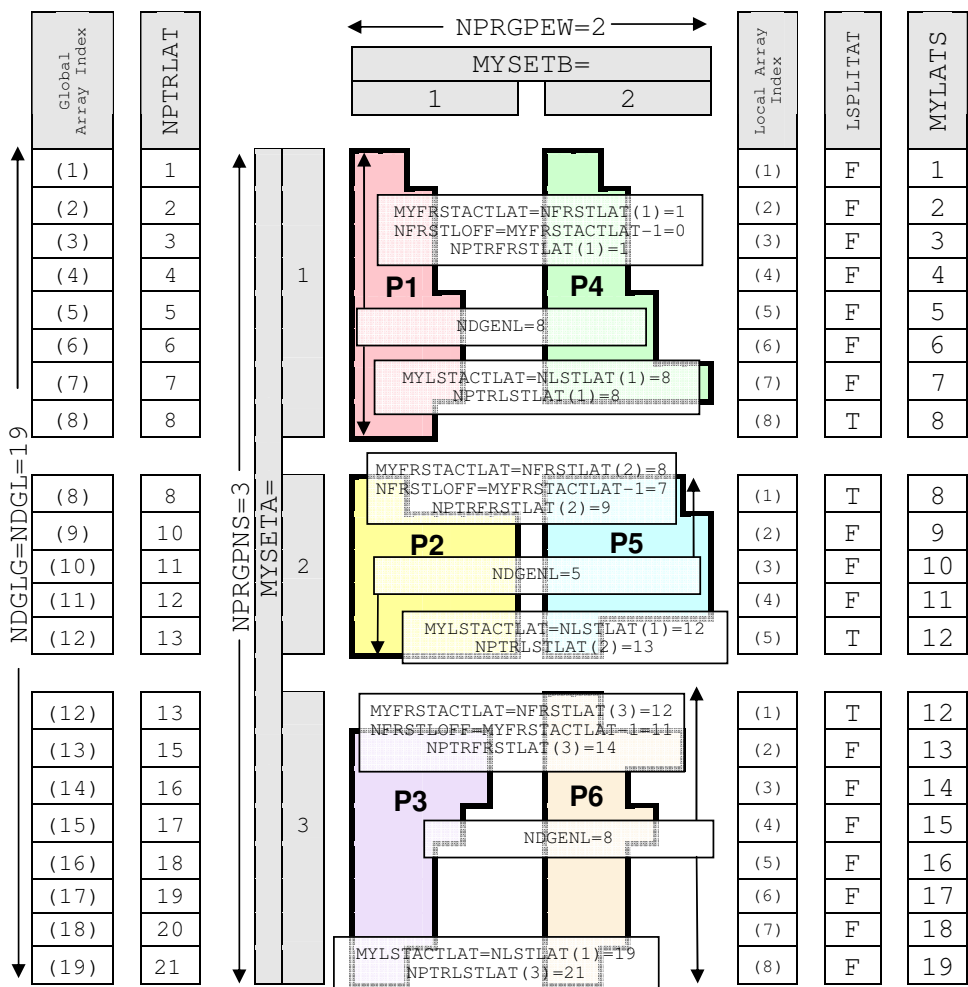
Figure 2.3 Variables describing the Grid Point Decomposition.
