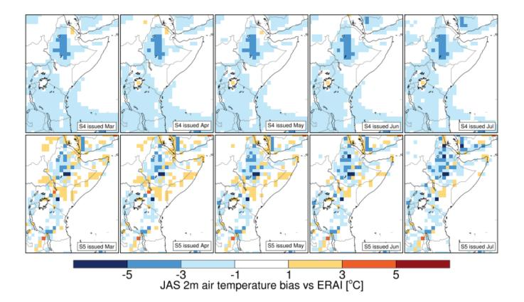
Figure 14. [BiasJAS] 2m temperature ensemble mean bias JAS, System 4 (top) and SEAS5 (bottom) vs ERAI
