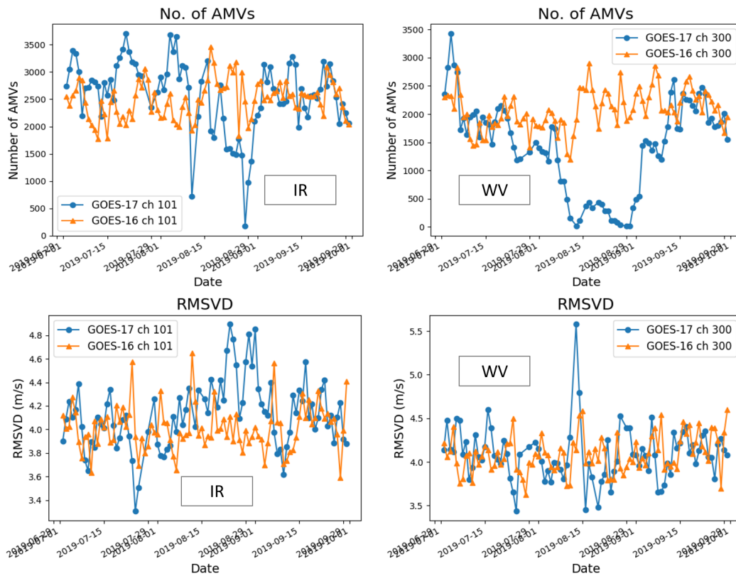
Figure 14: Top row: Timeseries of the daily average of the number of AMVs for actively used high level infrared AMVs (left) and water vapour AMVs (right) from GOES-17 and GOES-16. Bottom row: as above but for RMSVD. Data are for the period 1st July - 30th Sept for the hours 11-15Z only and from the experiment where no temporal screening is applied.
