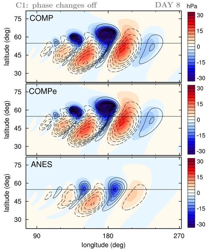
FIG. 1. Moist baroclinic instability with phase changes excluded at day 8, as simulated by COMP, COMPe and ANES models: surface virtual potential temperature perturbations (black isolines; c.i.=4 K; negative values dashed) and surface pressure perturbations (colored). Black lines at 53N mark the position of the zonal distributions shown in Fig. 2.
