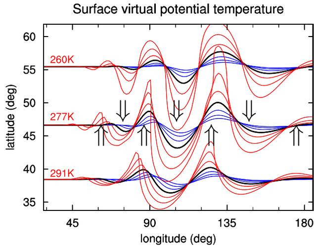
FIG. 7. Surface virtual potential temperature isolines for 260, 277, and 291 K at day 5.2 (black; start of the rapid growth of maximum  $\omega_s$ ), and 0.5, 1 and 1.5 day before/after that time (blue/red), for the COMP model (C3). The isolines were shifted zonally to fit those at day 5.2. The instability develops from zonally homogeneous  $\theta_v$ . The arrows mark the reciprocating meridional transports of relatively warm and moist (northward) and cool and dry (southward) air masses.
