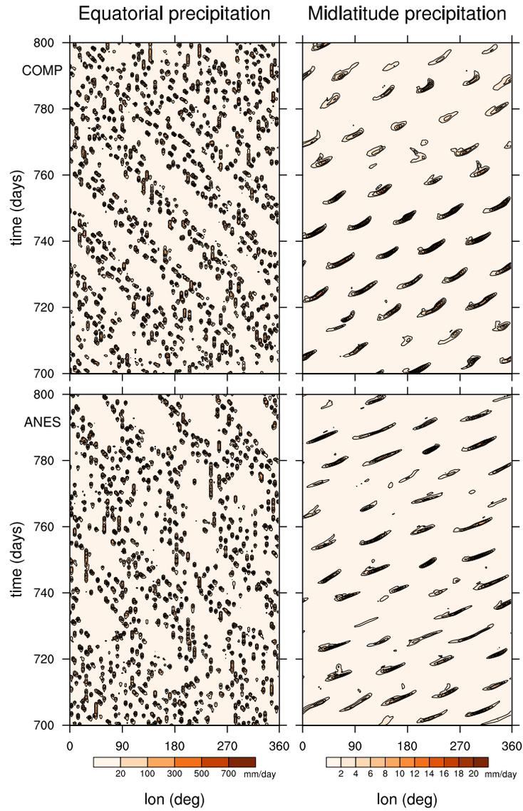
FIG. 17. Hovmöller diagrams of the surface precipitation for the tropics (left columns) and midlatitudes (55N, right columns) for COMP (upper panels) and ANES (lower panels) models, for the period of 100 days, starting from day 700.
