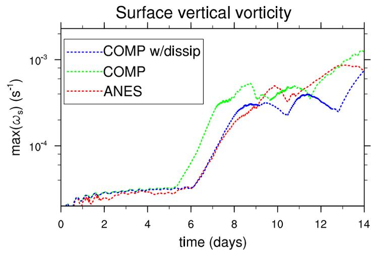
FIG. 19. History of the maximum surface vertical vorticity for COMP and ANES solutions (setup C3) from Fig. 6 together with the corresponding COMP solutions with heavy filtering in the advection scheme.
