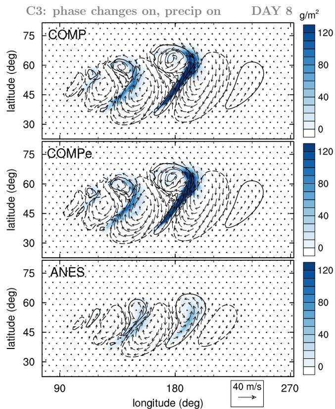
FIG. 3. Similar to Fig. 1 but with condensation and precipitation included. Cloud water path (colors) is plotted along with vectors of the surface horizontal winds. Black contours denote the  $-1/1$  K (dashed/solid) isolines of the surface virtual potential temperature perturbations.
